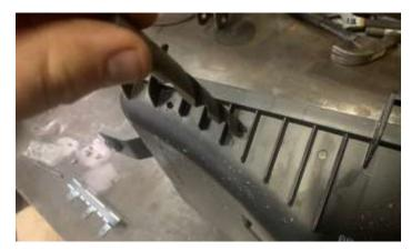
Deburr the 3 drilled holes by using a bigger drill. 10mm or thereabouts and just twist it by hand (it is only plastic after all) to take the burrs completely off, inside and out.
