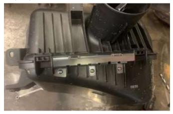
Test fit filter and lid, then reinstall airbox into vehicle. Easiest to do the base first, with the cable ties, then do the lid after. If you have any issues call us on (03) 9735 9099 or email sales@patrolapart.com.au
