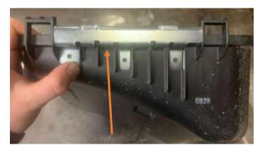
Remove the lid from the base if you haven't already and hold the Bracket up against the Air Box Base as pictured and mark out the 3 holes with a texta or similar. Make sure you hold the bracket right up against the top when marking out the holes, so the bracket sits against the shoulder. (arrow pointing up)
