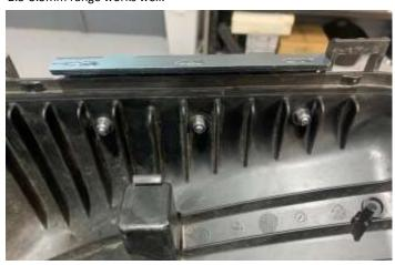
Fit the bracket as pictured, with the washers and nuts on the inside ensuring the bracket is pushed hard up against the shoulder as above.
