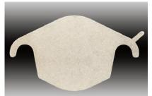
The EGR Block off plate replaces a gasket between the EGR Valve and intake manifold. To fit, remove the 2 EGR valve nuts that secures the EGR Valve to the manifold. It may be necessary to use some "penetrene on the nuts and allow to soak before undoing. Loosen the nuts enough to alow the blanking plate to slide betwen the valve and intake manifold. Re-fit housing and
