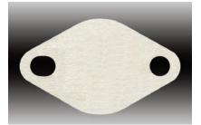
The EGR Block off plate replaces a gasket between the EGR Valve and intake manifold. To fit, remove plastic engine cover. Remove the two bolts that secures the EGR pipe to the manifold. It may be necessary to use some "penetrene" on the bolts and allow to soak before undoing. Remove the bolts to alow the blank-ing plate to slide betwen the valve and intake manifold. Re-fit housing and
