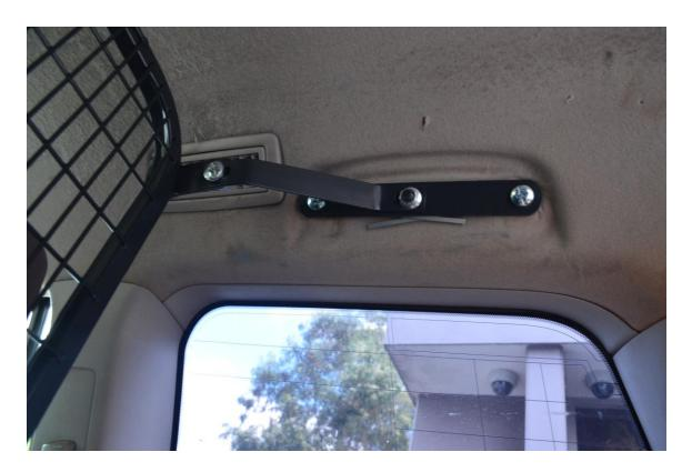
**BASE:** Remove the two luggage tie down points in the rear of the vehicle at 870mm centres, drill out the existing hole to 10mm. Secure one end of the 470mm straight bracket into the 10mm hole using an M10x30mm set screw and an M10 Mudguard washer on the underneath of the vehicle. (For maximum results, run a bead of silicone around the M10 mudguard washer before securing).
