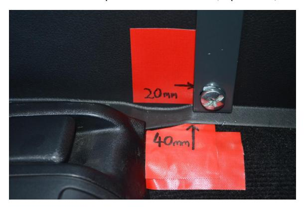
Hold the bracket in place (the flat edge of the bracket should be resting on the plastic).
