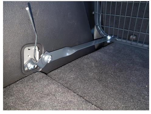
Attach the 29Z bracket to the M10 plate on wire thru the bottom hole of the plate with a M10x25mm set screw.
