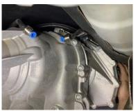
4. The Right Hand Hose running forward along the gearbox will become the New gearbox Breather. We Find it easiest to reach the gearbox breather fitting with the shift cable disconnected.
