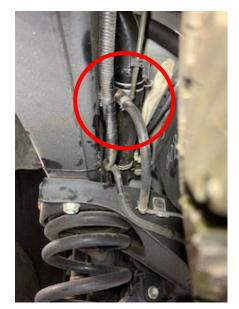
10. At the Rear of the Vehicle, you will find a metal pipe which runs in front of the spare tyre, below the fuel tank.
