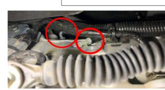
6. Connect both ends of the Supplied black breather pipe to the 2 Fittings you have installed and use the 2 supplied P Clamps to attach to the studs in the floor above the tail shaft keeping the lines as far from the exhaust as possible
