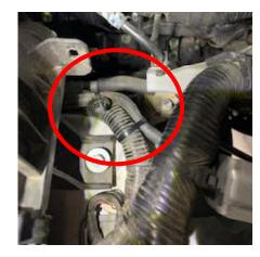
8. Run the 2 lines into the engine bay- between the Engine ecu and the Guard and cut to length
