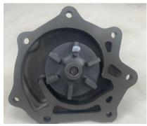
2. Fit the water pump to the timing case, with the gasket installed, and do up firmly. (we suggest using only the three bolts as circled in the picture below for test fitting).
