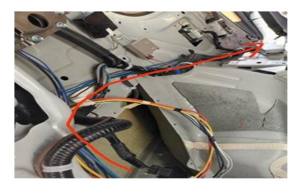
7. Run the Wiring Loom Towards the front of the vehicle alongside the factory wiring harness
