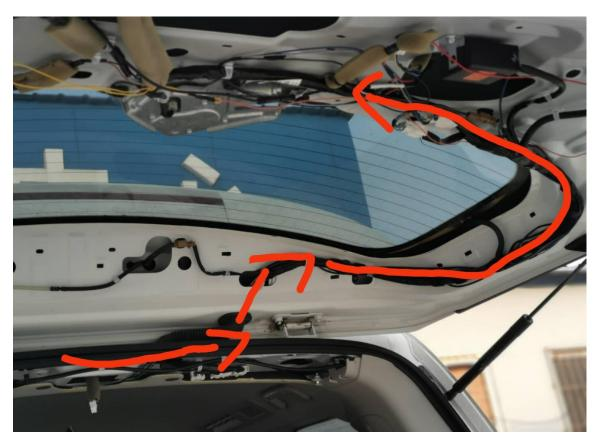
12. 7. Now run the Wiring loom from the Motor up to the Tailgate, Feed it through the factory tailgate boot and follow the path as outlined by the red line
