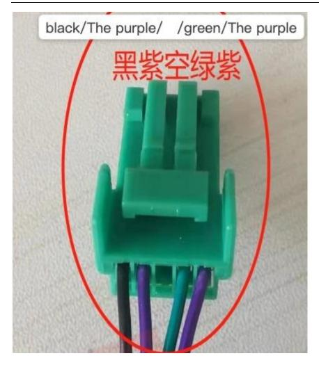
14. Fit off the Connector for the Tailgate swith
