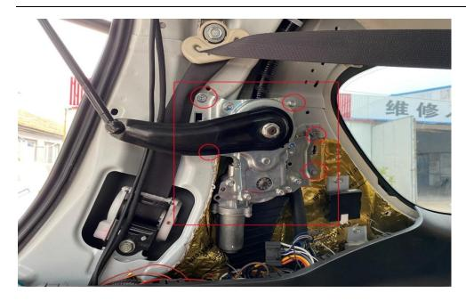
6. There are four screw holes which are used to fix the motor on the D-pillar and side plate. The motor should be fixed as shown in the picture.
