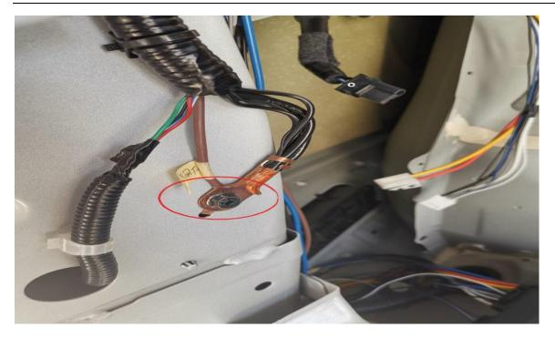
8. Connect the ground/Earth wire to the original car D-pillar main ground line.
