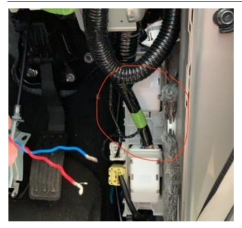
10. Run the wiring Harness under the dash to the RH side of the car, remove the RH Kick Panel and lower Dash trim to gain access. Trim back the plastic on this wiring loom and Join/Solder the Red/Blue Twisted can wires in the supplied harness to the Pink/Blue (Series 1-3) or Red/Blue (Series 4-5) twisted wires in
