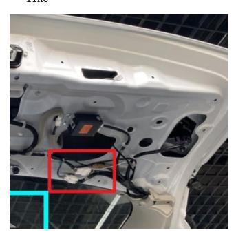
13. Plug in the Patch Loom for the tailgate harness.
