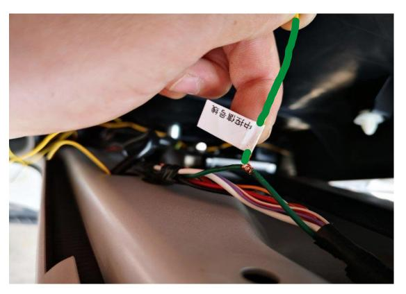
9. Remove the B-pillar trim panel, and connect the green central control unlocking Wire in the Vehicle's Wiring Loom, to the Green central control Signal Wire In the supplied harness for the Tailgate
