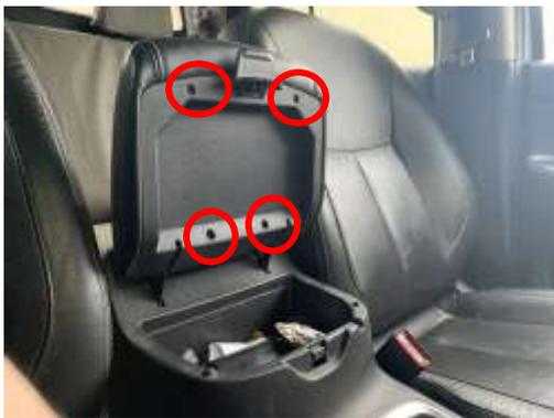
2. Once all screws are removed gently pry the plastic base/trim off the underside of the console lid.
