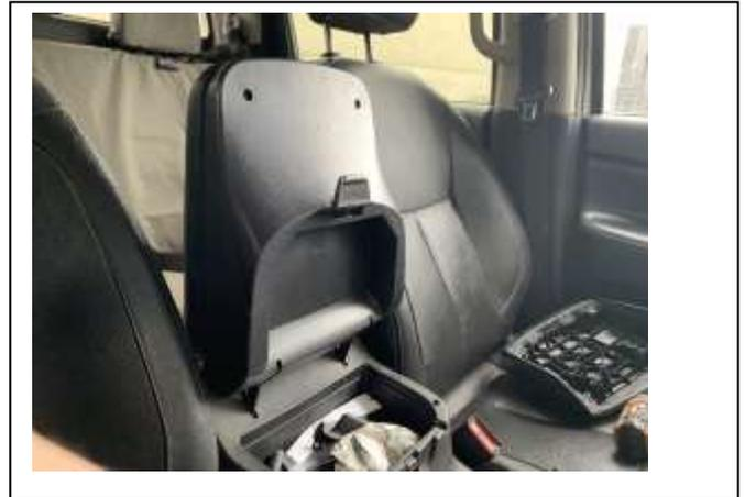
9. Ensure the Console Latch, latches properly and releases easily. The spring should hold it in the closed position.
