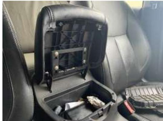
3. Remove the 4 Silver Phillips head screws Holding the Console Lid to the metal frame and remove the console lid from the frame.
