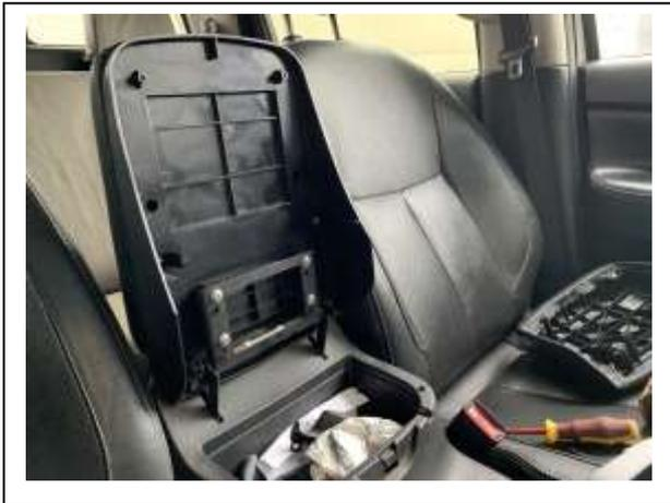
8. Fit the Console lid Lower Trim (with the latch installed) and re-fit the 6 black Phillips head screws previously removed.
