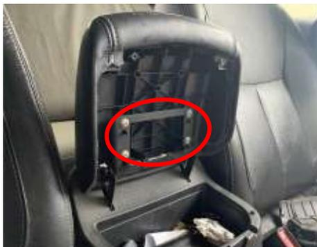
4. Remove the 6 screws holding the plastic base plate to the new console lid, and gently pry off to separate the console lid into 2 halves.
