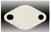
The EGR Block off plate replaces a gasket between the EGR Valve and intake manifold. To fit, remove plastic engine cover. Remove the two bolts that secures the EGR pipe to the manifold. It may be necessary to use some "penetrene" on the bolts and allow to soak before undoing. Remove the bolts to alow the blank-ing plate to slide betwen the valve and intake manifold. Re-fit housing and tighten all bolts.
