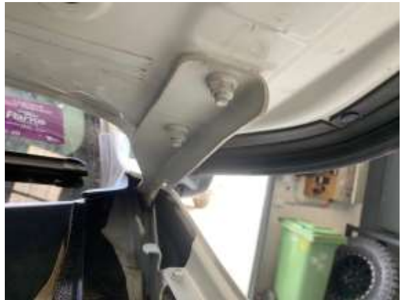
Remove these two nuts carefully while holding the bonnet, so it doesn't come off the hinge.
