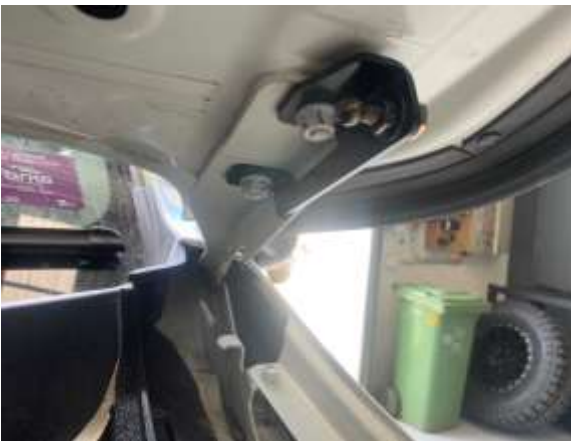
Install bracket with the top stud facing inwards
