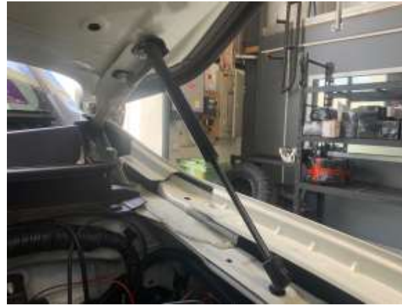
Clip Strut in, with the body at the top side, and repeat process on the other side of the car. Happy Days!
