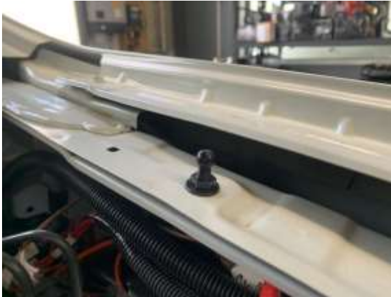
Install bottom stud with the large zinc washer underneath the inner skirt and tighten.
