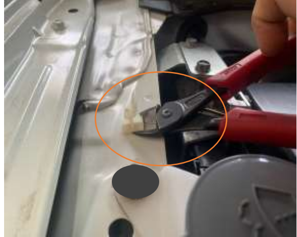
Cut support rod carrier clip or unclip from skirt.
