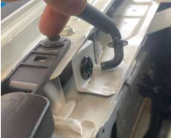
Remove the bonnet support rod by twisting out.
