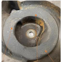
You can see the ripples in the once smooth timing cover, caused by cavitation. These continue to create cavitation.
