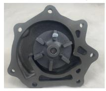
Using both gaskets in tandem, fit the water pump to the timing case, and do up firmly (we suggest using only the three bolts as circled in the picture below for test fitting).
