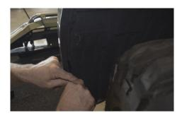
8. Pull away the wheel liner to unbolt the bumper from the front quarter panels.
