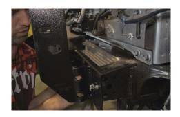
18. Make up the support bracket and fit to the chassis as shown. See the second photo to ensure that the support brackets are fitted correctly.
