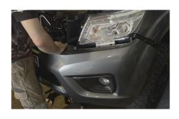
10. Remove the plastic mouldings underneath the headlights.
