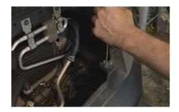
6. Undo the bolts holding the lower part of the bumper as shown.
