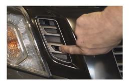
4. Pull the grill away, pushing the clips where it attaches to the bumper.
