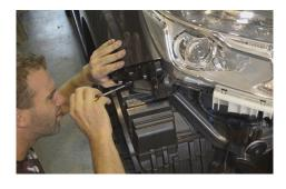
11. Unbolt and remove the front impact bar.
